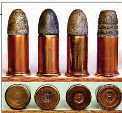
These four different .44 Henry cartridges were made back in the 1800s. The first three rounds have early-style pointed bullets without any exterior grooves.
